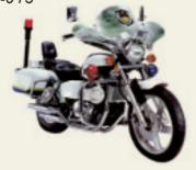
**Technical parameter** Length\*Width\*Height: 2270mm\*900mm\*1080mm Wheelbase: 1465mm Rated load quality: 160kg Maximum speed: 100km/h Wheel felloe style: Light alloy Writer Trie (front/back): 90/90-18, 130/90-15
